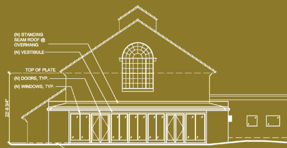
12 EXTERIOR ELEVATION @ SOUTH WALL - MAIN HALL SCALE: 1/8" = 1'-0"
